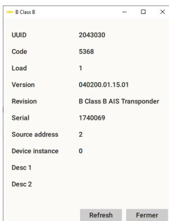
By clicking on an instrument, you have access to more detailed information about it. For the **Box N2K**, it is possible to modify some parameters: NMEA 2000 address, Instance, and description fields.
