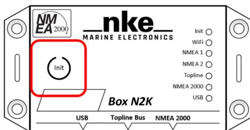
When the Init button is pressed, the "Init" indicator lights up green and a beep is heard every second to facilitate counting.
