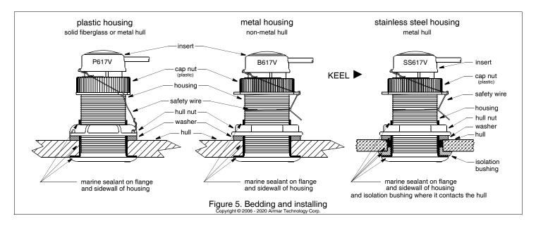
Stainless steel housing in a metal hull—A stainless steel housing must be isolated from a metal hull to prevent electrolytic corrosion. Slide the isolation bushing onto the housing. Apply additional sealant to the surfaces of the isolation bushing that will contact the hull, filling any cavities in and around the bushing.
