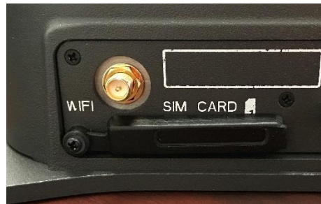
Figure 2-14 Secure the SIM Card Cover
