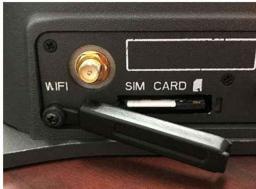
Figure 2-12 SIM Card with Cover Opened
