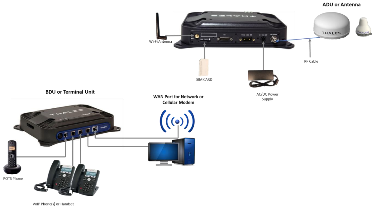
Figure 2-3 Thales VesseLINK™ System with Accessories
