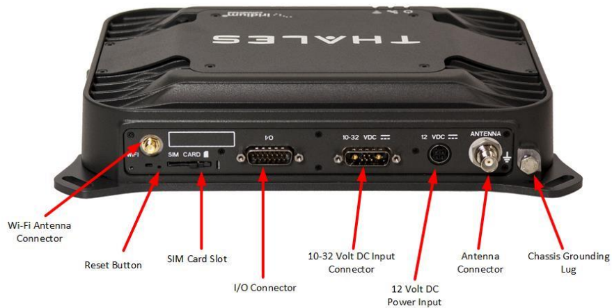
Figure 2-7 Below Deck Unit (BDU) Back Panel Detail
