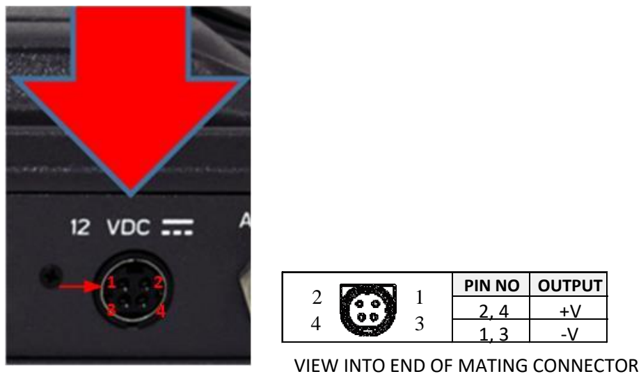
Figure 7-3 12V Input and Mating Connector Detail
