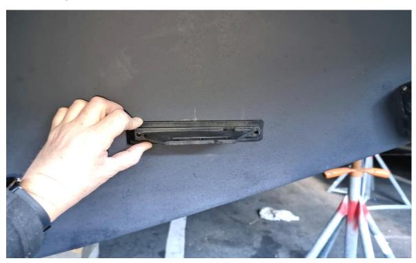
**STEP 3:**Drill holes for the motor bracket, use 5mm drill bit, then use the 6mm threading loss and make treads in the holes
