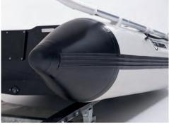
**Rubbing strake** Rubbing strake around the boat which protect the tubes.
