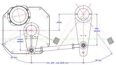
The direct drive uses "wide angle geometry". The result of this is 128° travel of the output lever and 72° travel of the tiller lever. To achieve an equal travel of the drive in port and starboard, the centre point of the output lever needs an offset to the rudderstock centre. The offset depends on the used lever centres. Following table shows the correct offset distances:
